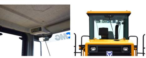
Fully-covered exquisite interiors, processed cab and hood by damping noise reduction, reduce the noise by over 6dB and build best operation environment.
